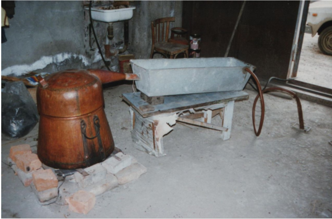
Figure 2.3. A traditional device for alcohol distillation in Kakheta, Georgia ( https://commons.wikimedia.org/w/index.php?curid=4462903 )
